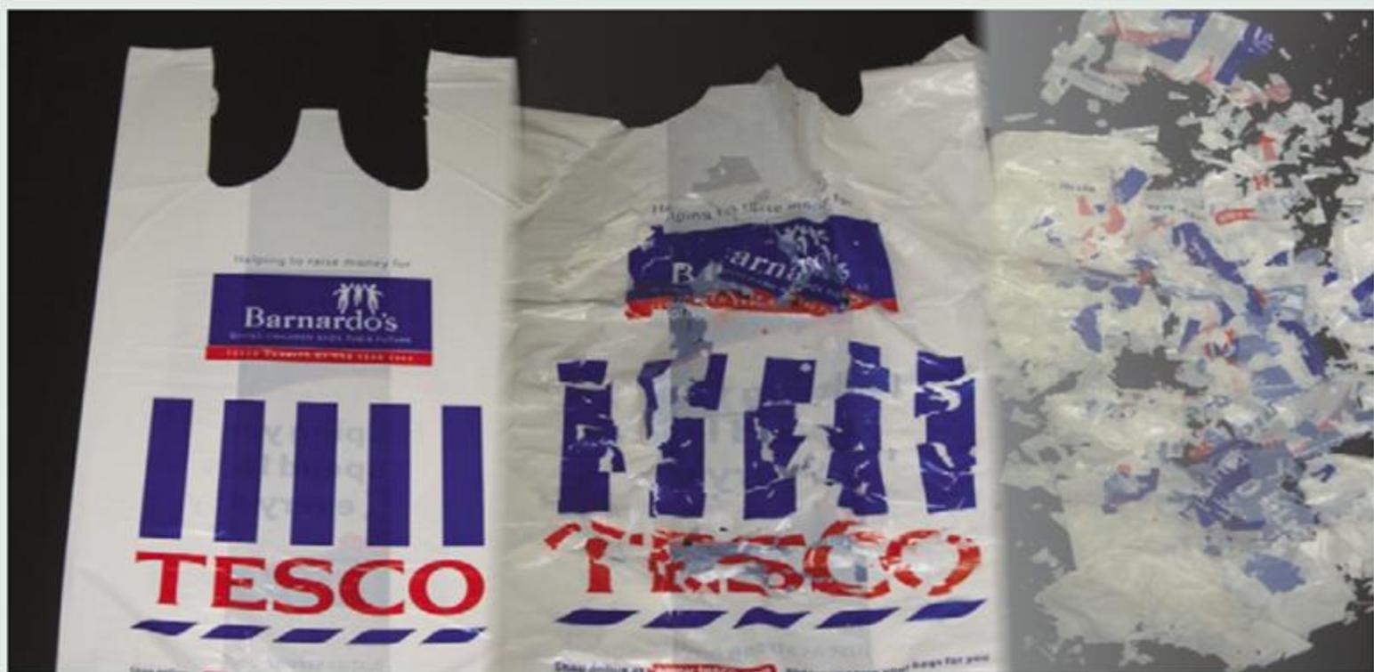
*This series of photos shows the stages of degradation possible using EPI degradable additives.*
